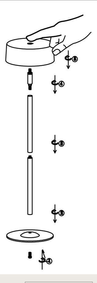
Do not tighten screws until all screws have been assembled!
