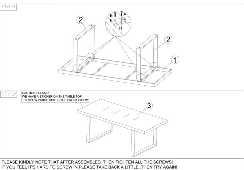
Do not tighten screws until all screws have been assembled!
