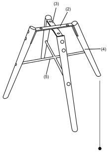
After leg completely assembled, please be sure to put the leg on the flat floor or glass platform to check if the leg is assembled well of not. If only 2 pcs of le touched the floor, please according to the photo showed and use your hand to adjust the leg which touched the floor and to make sure 4 pcs legs at the same level
