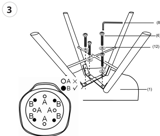
After leg completely assembled, please be sure to put the leg on the flat floor or glass platform to check if the leg is assembled well or not. If only 2 pcs of leg touched the floor, please according to the photo showed and use your hand to adjust the leg which touched the floor and to make sure 4 pcs legs at the same level
